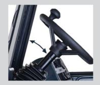
> Tilt adjustable steering for optimum operator interface
