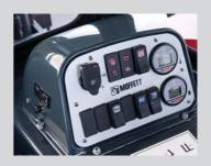
> M-series dash panel, with IP65 gauges / switches
