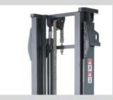
> Heavy duty standard 4 Mast, adjustable wear pads, pivot forks and option of Rotator
