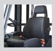
Fully adjustable air suspension seat for operator comfort
