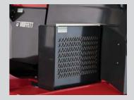
> High capacity hydraulic Oil Cooler
