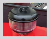
> The air filter pre-cleaner helps keeping feathers and dust out of the air filter The operator compartment is fully enclosed with toughened glass panels for winter use and can be easily removed for open air use during warm weather months.
